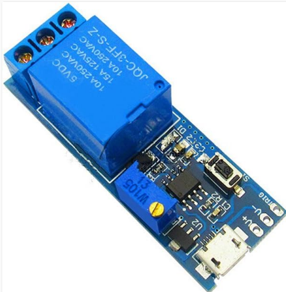
Figure 1: Top view of the Lianshi Multifunction Delay Time Module. This image displays the module's components including the micro USB power input, the blue potentiometer (W105) for delay adjustment, the onboard trigger button (S1), and the blue relay with its specifications (5VDC, 10A 250VAC, 15A 125VAC, 10A 250VAC, JQC-3FF-S-Z). Screw terminals for output connections are visible on the right.
