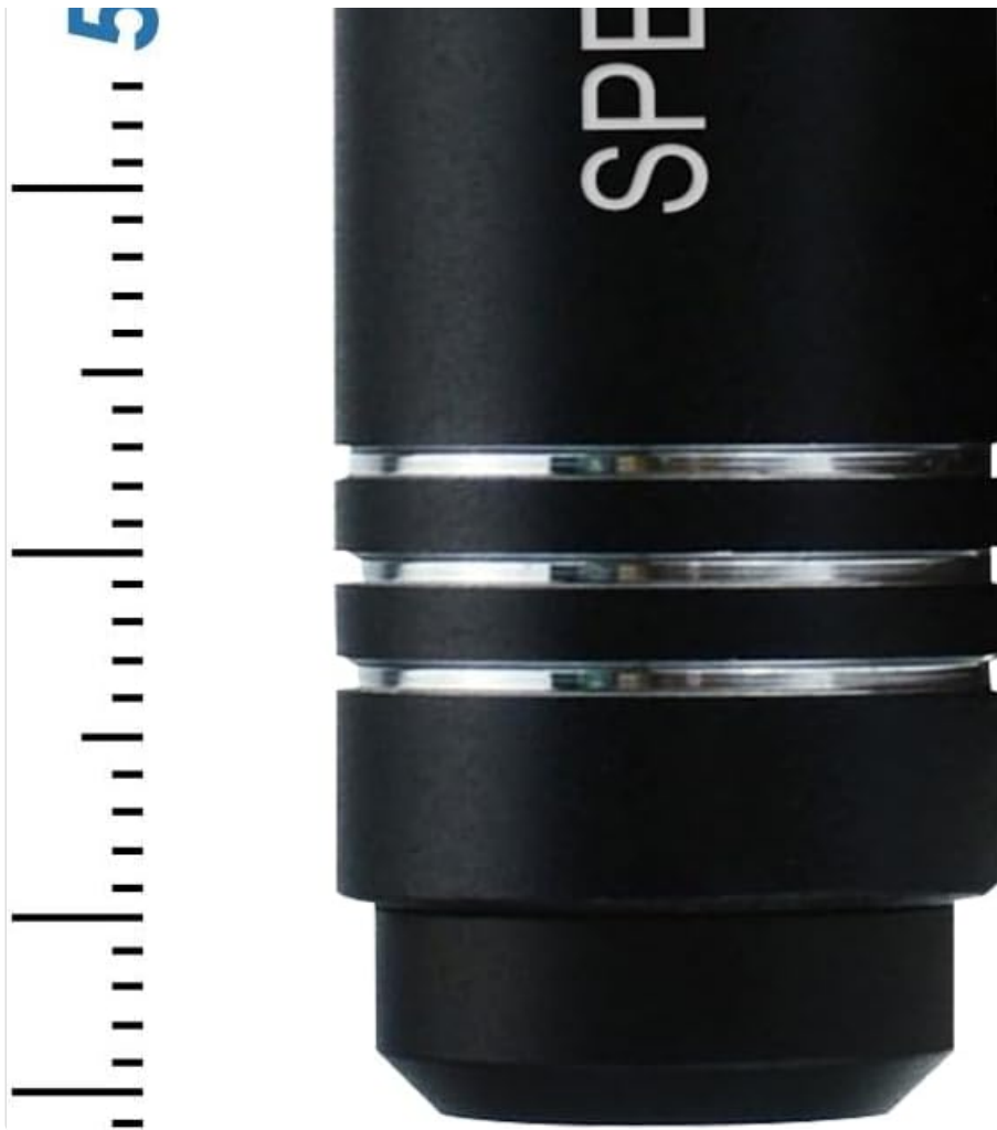
Figure 7.1: A visual representation of the spectroscope's dimensions, indicating its length of 55mm and diameter of 18mm at its widest point.
