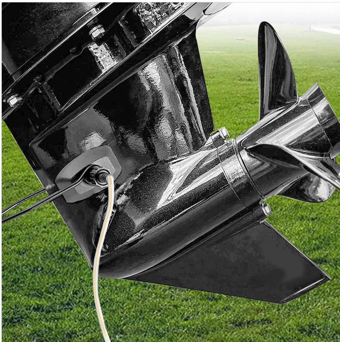
Figure 3: The water flusher correctly installed on an outboard motor's water intake.
