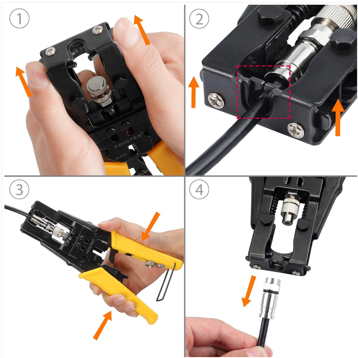
Image: A four-panel image illustrating the process of inserting a cable into the crimper, compressing the connector, and removing the finished crimped cable.
