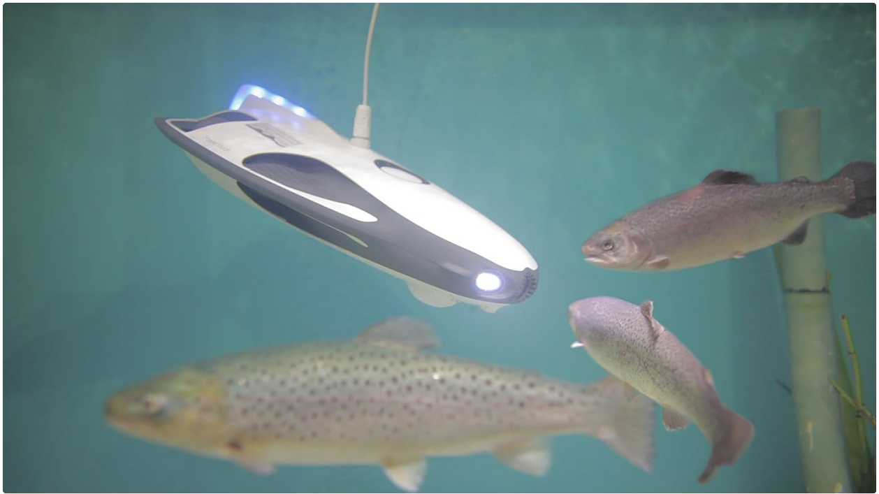
Figure 3.3: The PowerRay Wizard interacting with fish, showcasing its utility for fish finding and observation.
