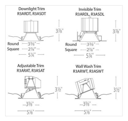
This diagram provides detailed dimensions and visual representations of various WAC Lighting Aether trim types, including Downlight, Invisible, Adjustable, and Wall Wash, with their respective cutout and aperture sizes.
