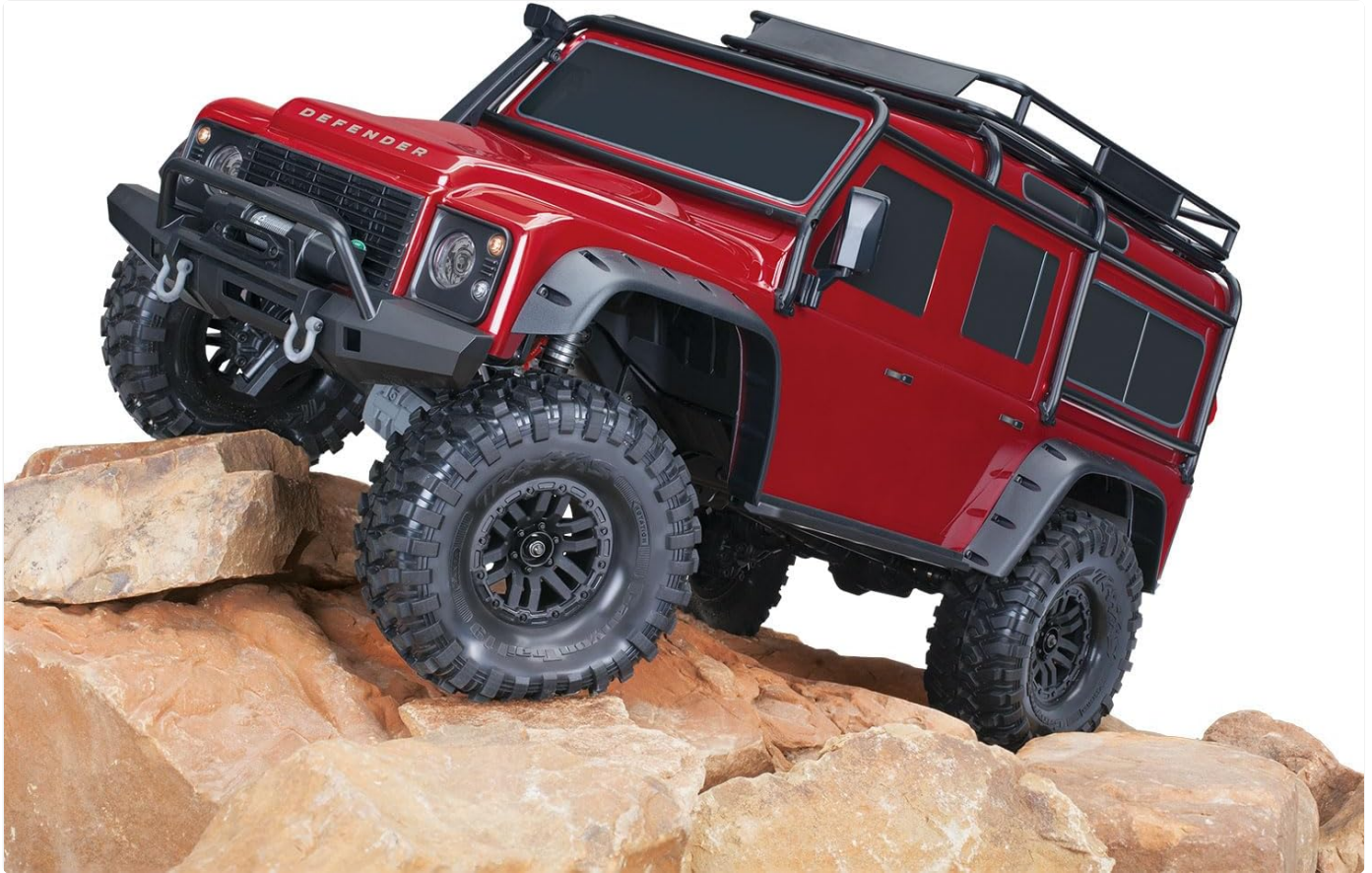
Figure 3: The TRX-4 demonstrating its climbing capabilities on rocky terrain, highlighting its portal axles and high ground clearance.
