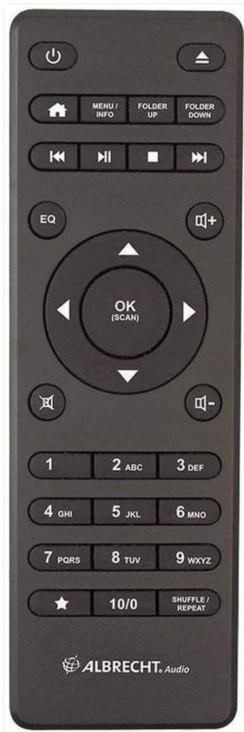
Figure 1.3: The included remote control for the Albrecht DR 890 CD. It features buttons for power, menu navigation, volume, playback control, source selection, and numerical input for direct access.
