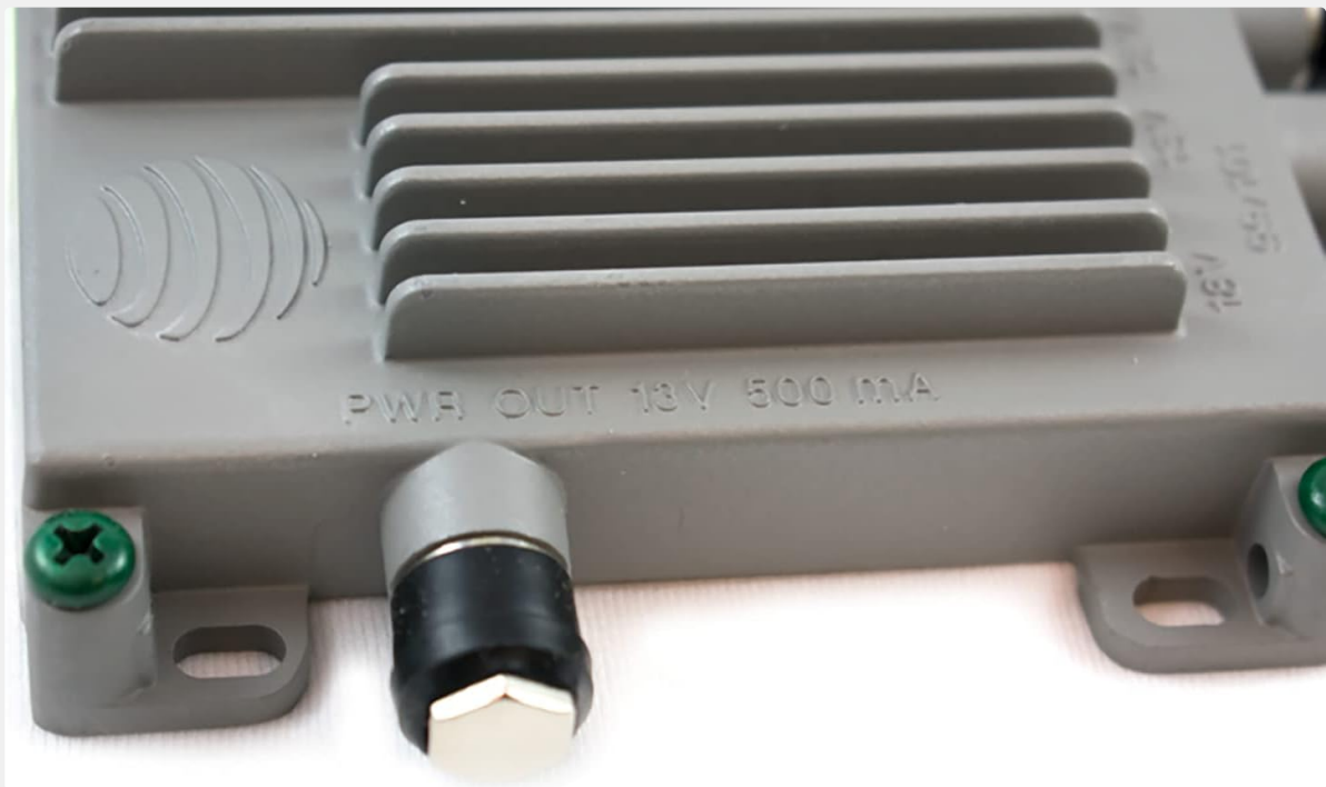
Figure 4.4: Close-up of the PWR OUT 13V 500mA port, indicating its capability to power coax-powered devices.
