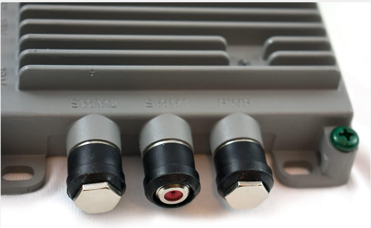
Figure 4.3: Detailed view of the SWM1, SWM2, and PWR output ports, where SWM-capable receivers connect and power is injected.
