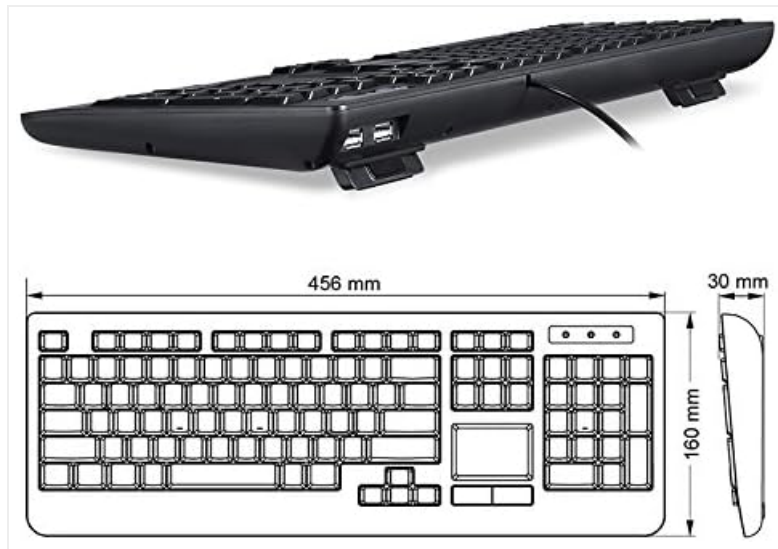
Image: Technical drawing with key dimensions of the PERIBOARD-313 keyboard.
