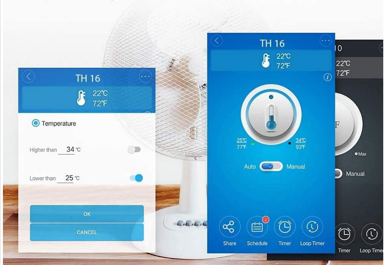
Image 4: The eWeLink app demonstrating the selection between automatic and manual control modes for the TH10 switch, with temperature settings for automation.
