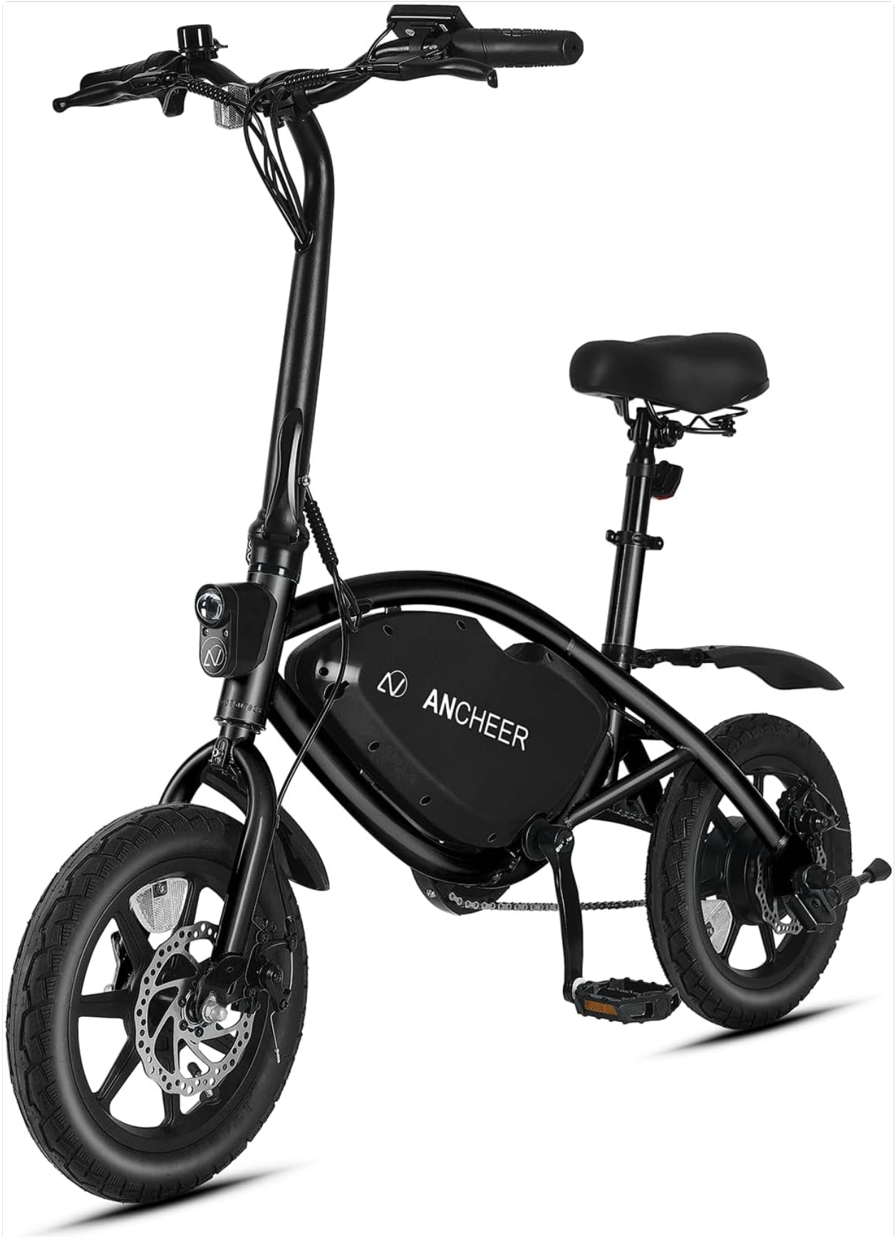
Image: A full view of the ANCHEER 14-inch Folding Electric Bike in black, showcasing its compact frame, integrated battery, and disc brakes.
