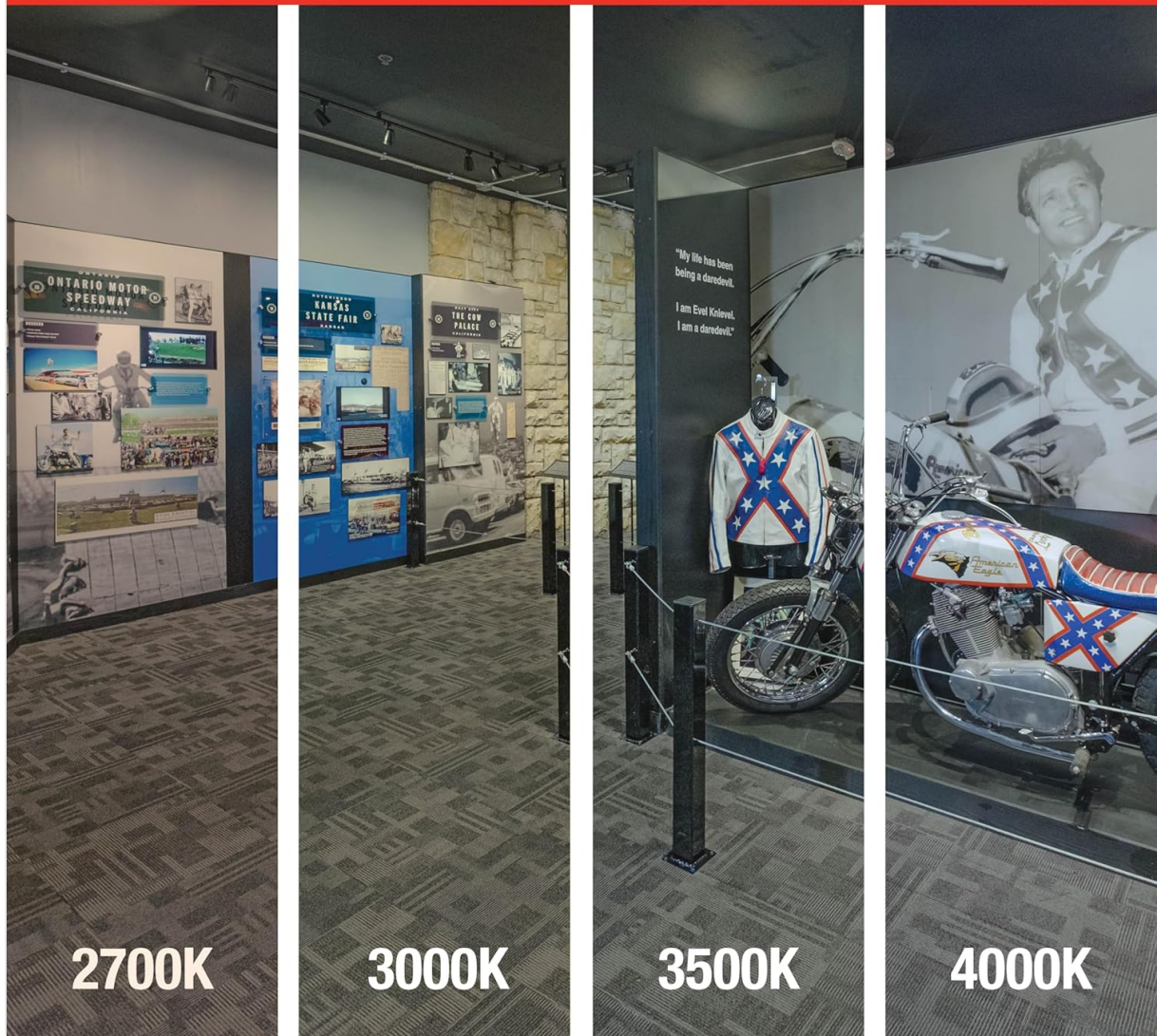
Figure 5: Visual guide demonstrating different color temperatures (2700K, 3000K, 3500K, 4000K) and their appearance in a display setting.
