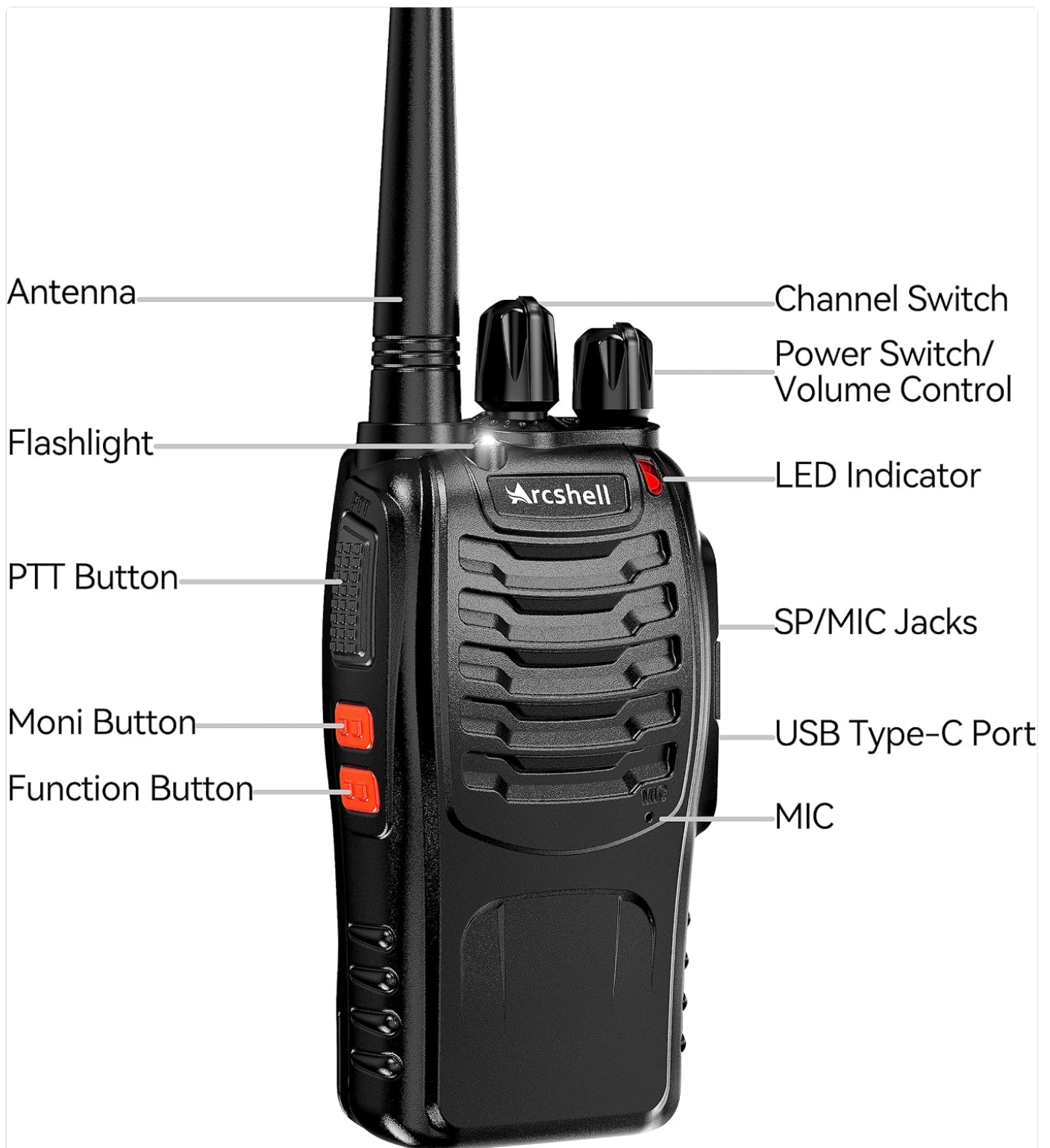
Figure 5: The USB Type-C charging port on the Arcshell AR-5 radio.
