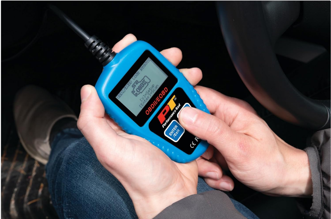
Figure 4: The W2976 scanner connected to a vehicle's OBDII port, ready for operation.
