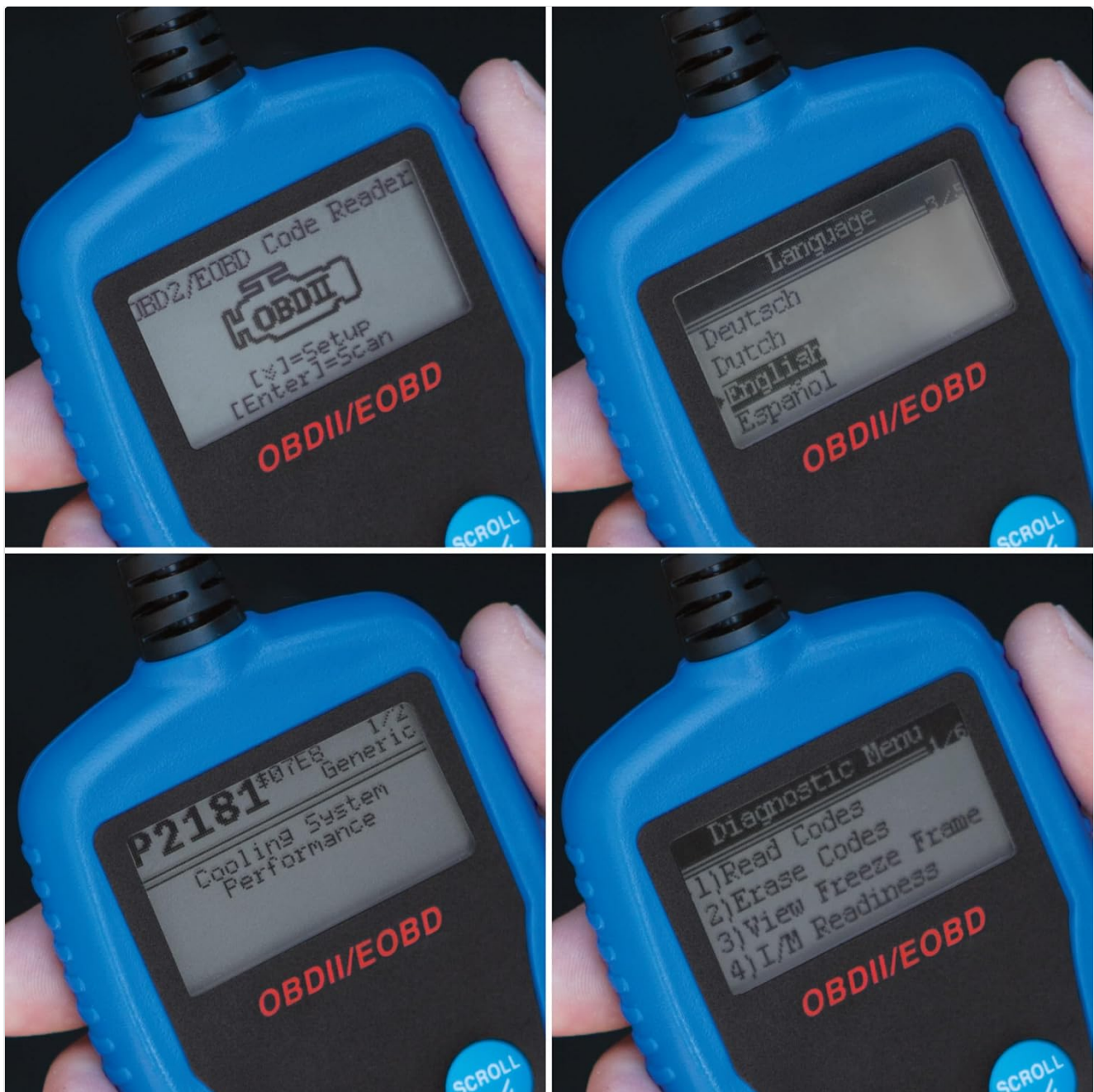
Figure 5: The scanner's display showing a diagnostic menu and an example trouble code (P2181).
