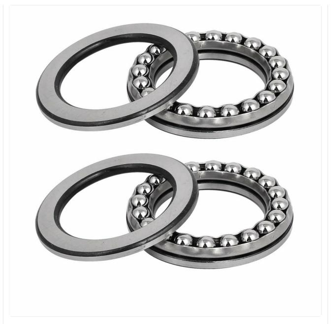
Figure 1: Two assembled uxcell 51108 Thrust Ball Bearings. Each bearing consists of a shaft washer, a housing washer, and a ball and cage assembly.
