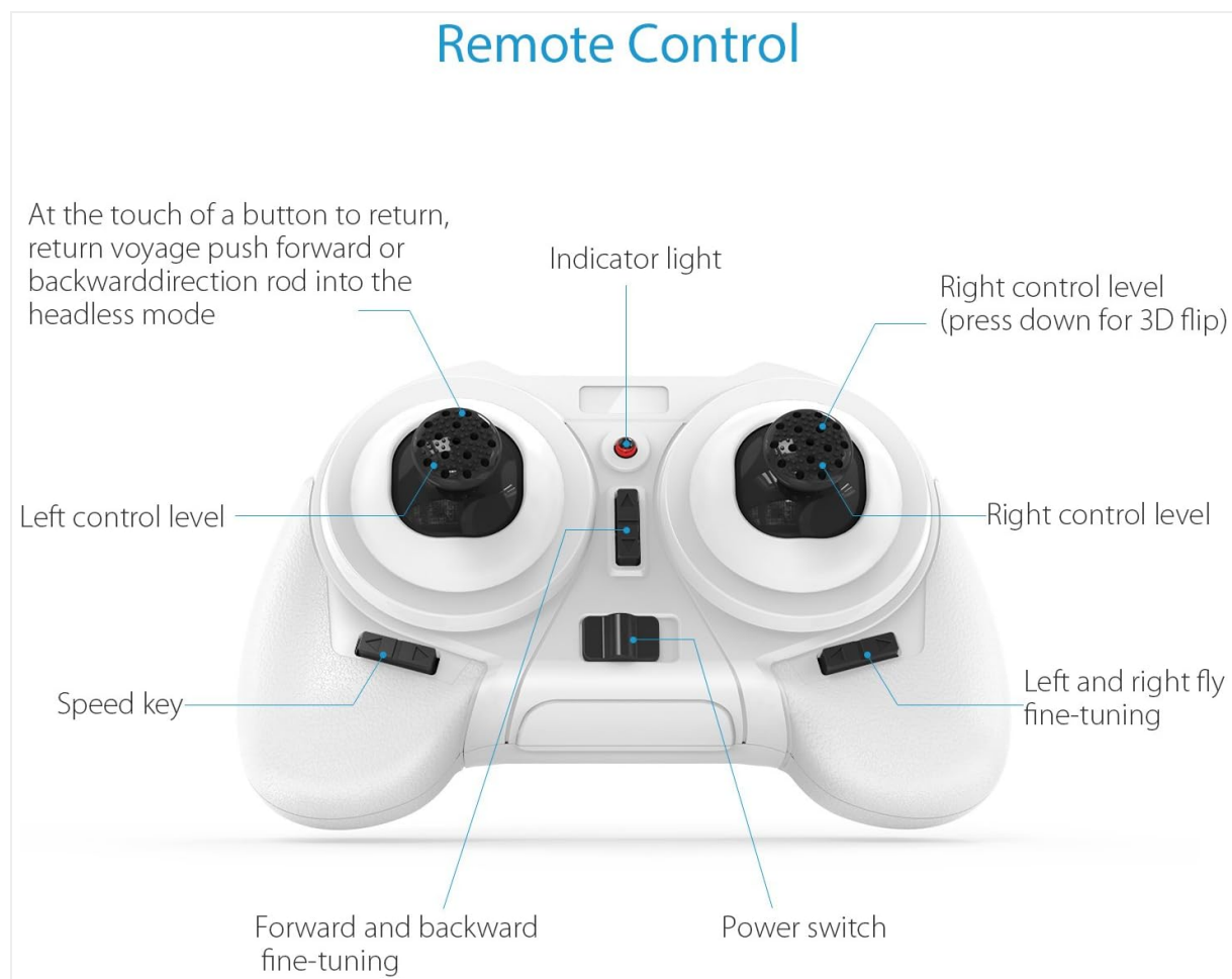
Image: Labeled diagram of the remote control for the GoolRC T36 drone.
