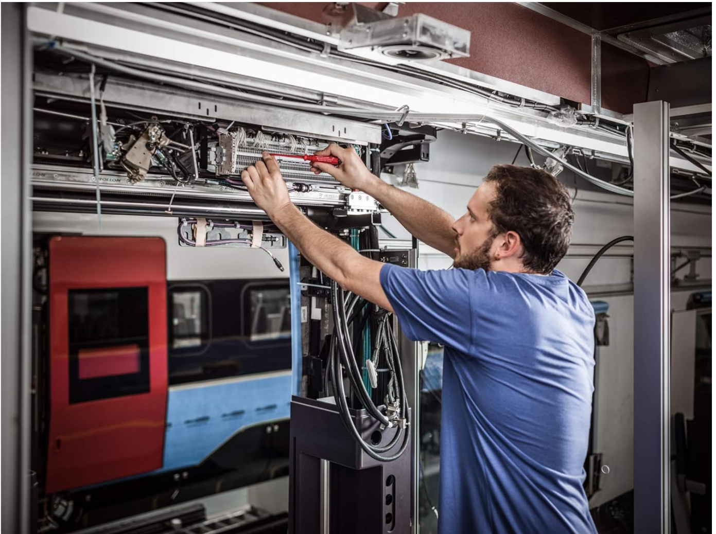
Image 3.2: A technician working with a precision screwdriver on intricate wiring and components within a train's interior, highlighting the tool's suitability for detailed electrical work.
