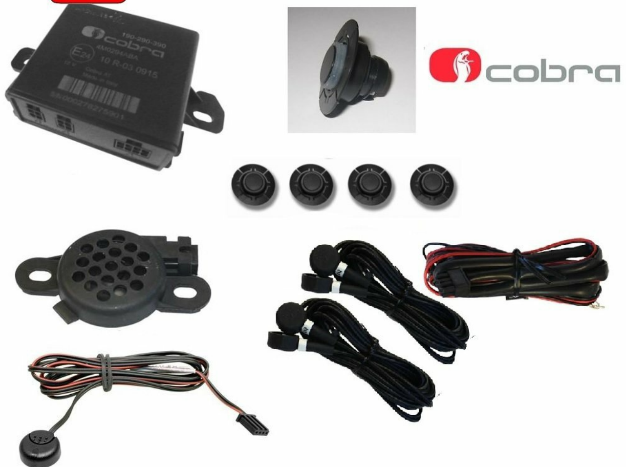
Image 2.1: Overview of the Cobra F394 front parking sensor kit components.
