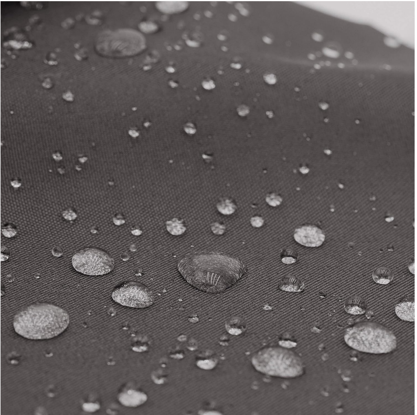
Image 6.1: Waterproof fabric showing water beading.
