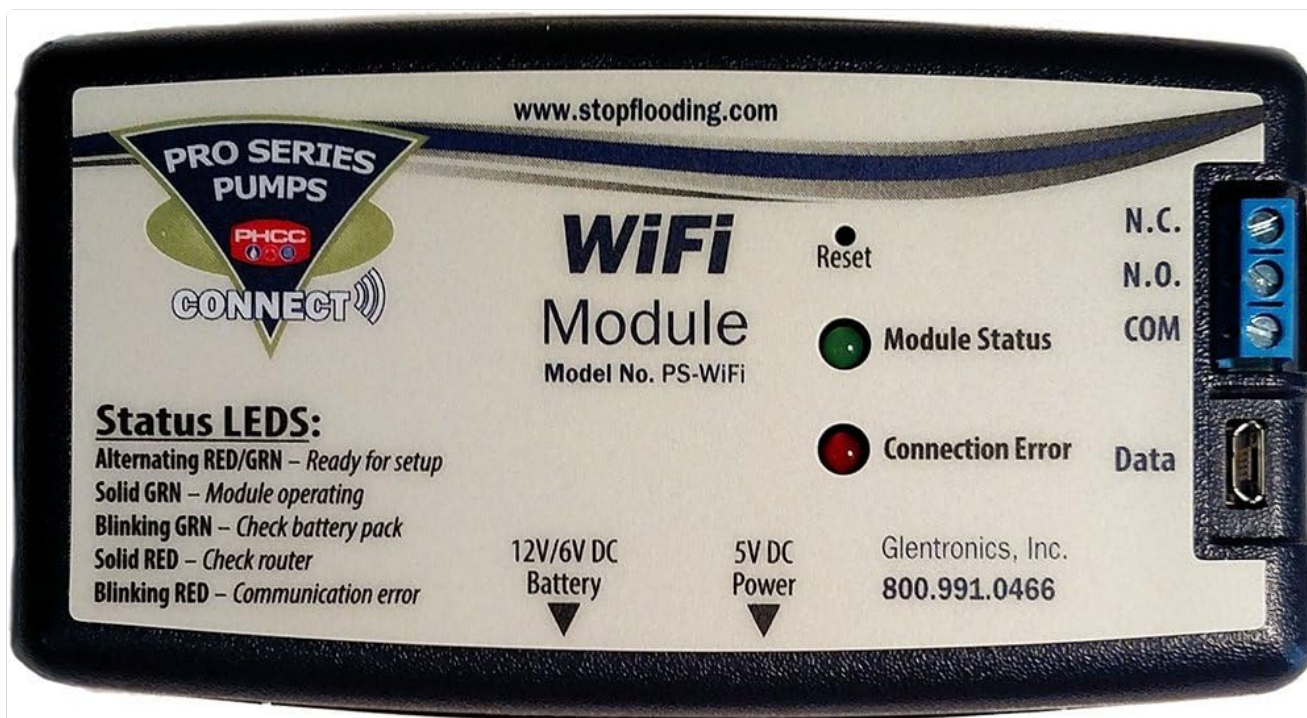
Figure 1: The Pro Series WiFi Module, a black rectangular device with labels for 'WiFi Module', 'Model No. PS-WiFi', 'Reset button', 'Module Status LED (green)', 'Connection Error LED (red)', 'N.C.', 'N.O.', 'COM' terminals, 'Data port', '12V/6V DC Battery input', '5V DC Power input', and 'Status LEDs' descriptions.
