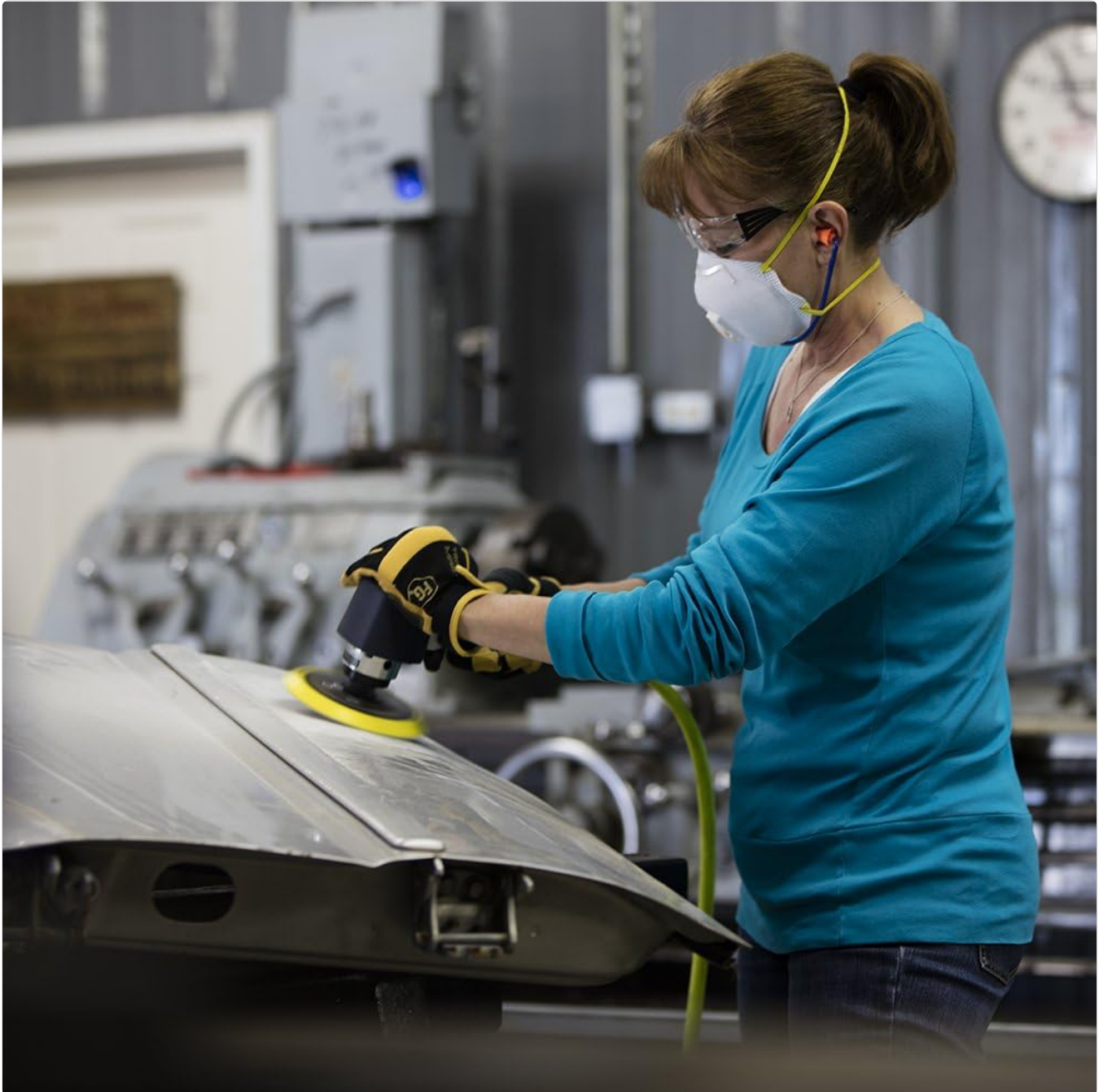
Figure 5.1: An individual utilizing an air-powered orbital sander, connected to an air compressor via a hose. This demonstrates a typical application for the compressor in a workshop setting, highlighting the use of air tools for tasks like surface preparation.
