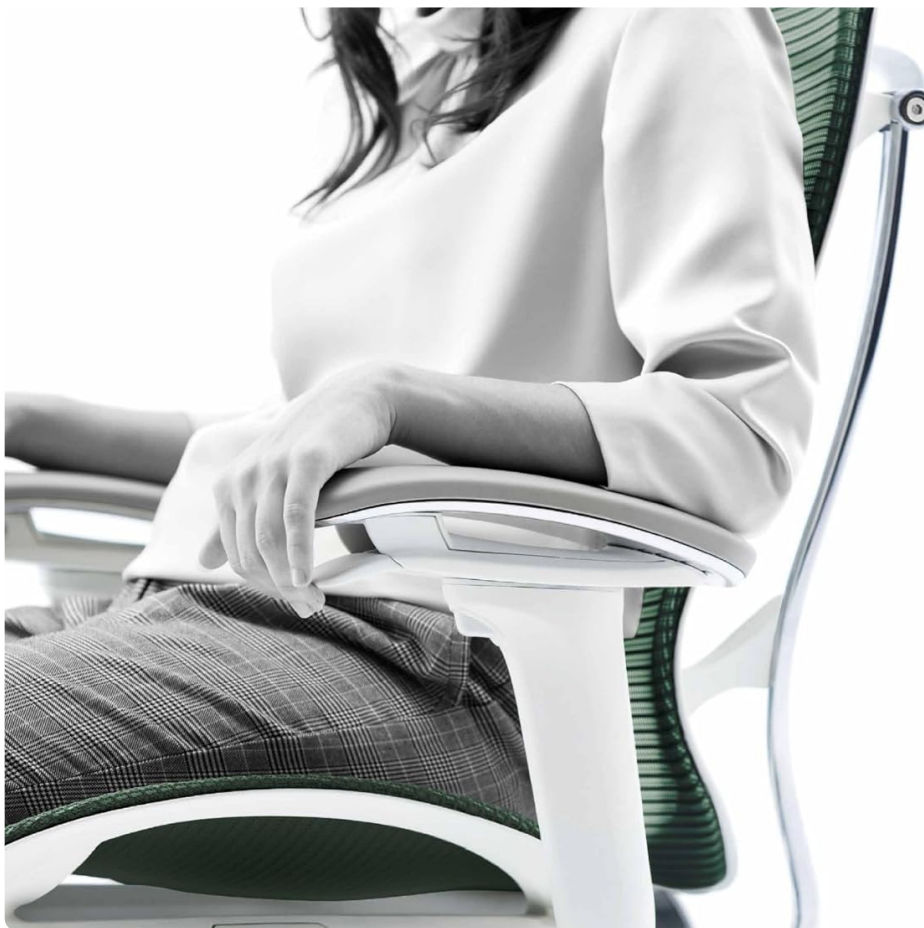
Figure 6: The armrests offer 4-dimensional adjustments: up/down (1D), angle (2D), forward/backward (3D), and left/right (4D). The angle can be adjusted 15 degrees inward and 7.5 degrees outward. The armrest pads can also be moved 25mm left or right.
