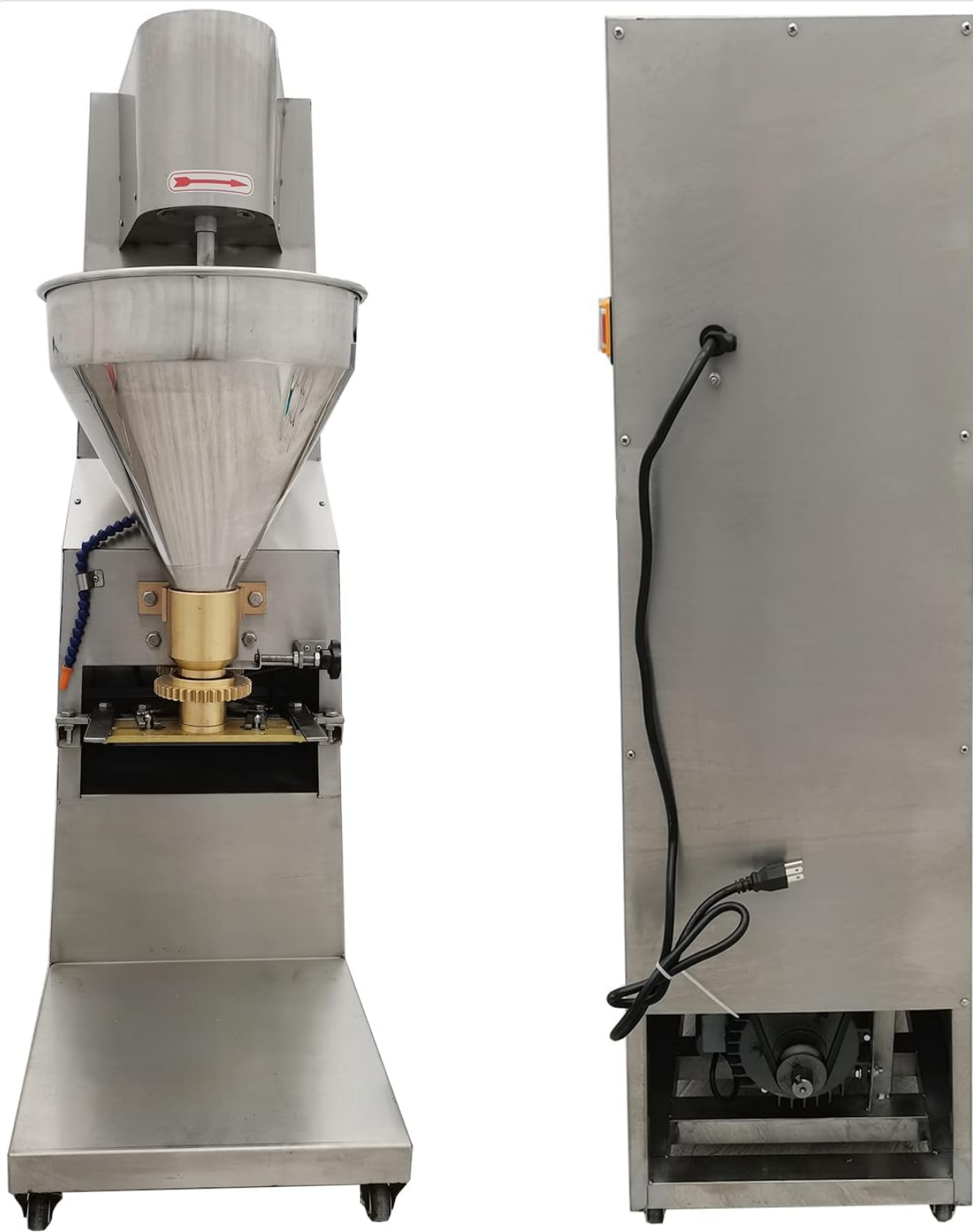
Figure 3.2: Front and back views of the machine, highlighting the hopper, forming mechanism, and power cord connection.
