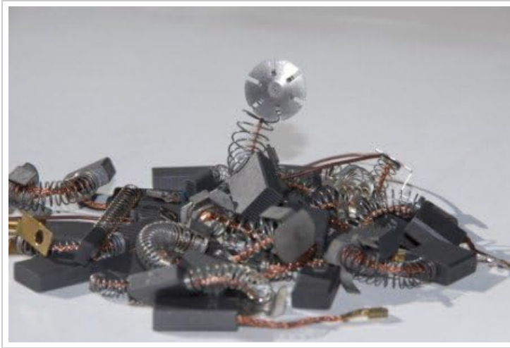
Figure 6.1: A collection of carbon brushes and associated motor components. Regular maintenance helps identify worn parts before they cause tool failure.
