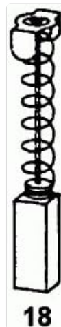
Image 2: Diagram illustrating the components of a carbon brush, including the carbon block, spring, and cap.
