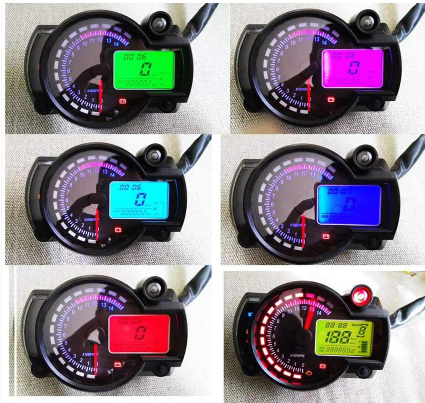
Image 6.2: Examples of the speedometer display with different backlight color options.
