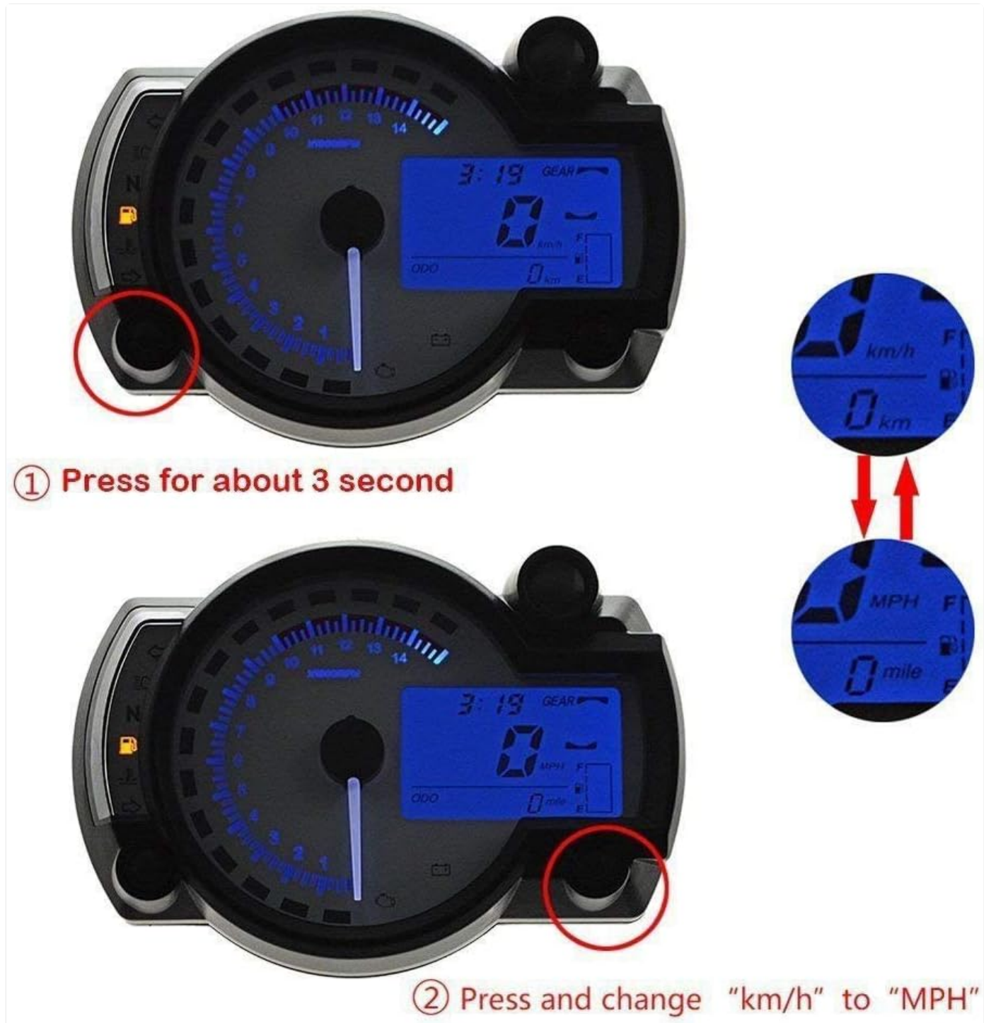
Image 6.1: Visual guide for changing the speed unit from km/h to mph by pressing and holding the button.
