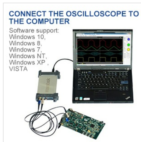
Image: A visual guide demonstrating the connection of the Hantek 6022BE oscilloscope to a laptop computer via USB, illustrating the PC-based nature of the device.
