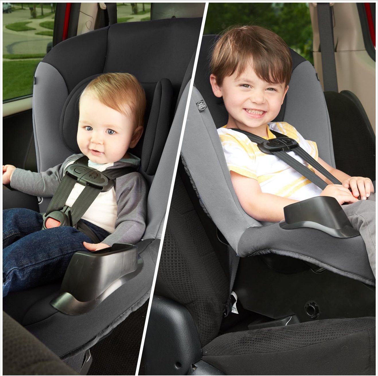
Figure 4.1: Comparison of rear-facing (left) and forward-facing (right) child positions in the car seat.
