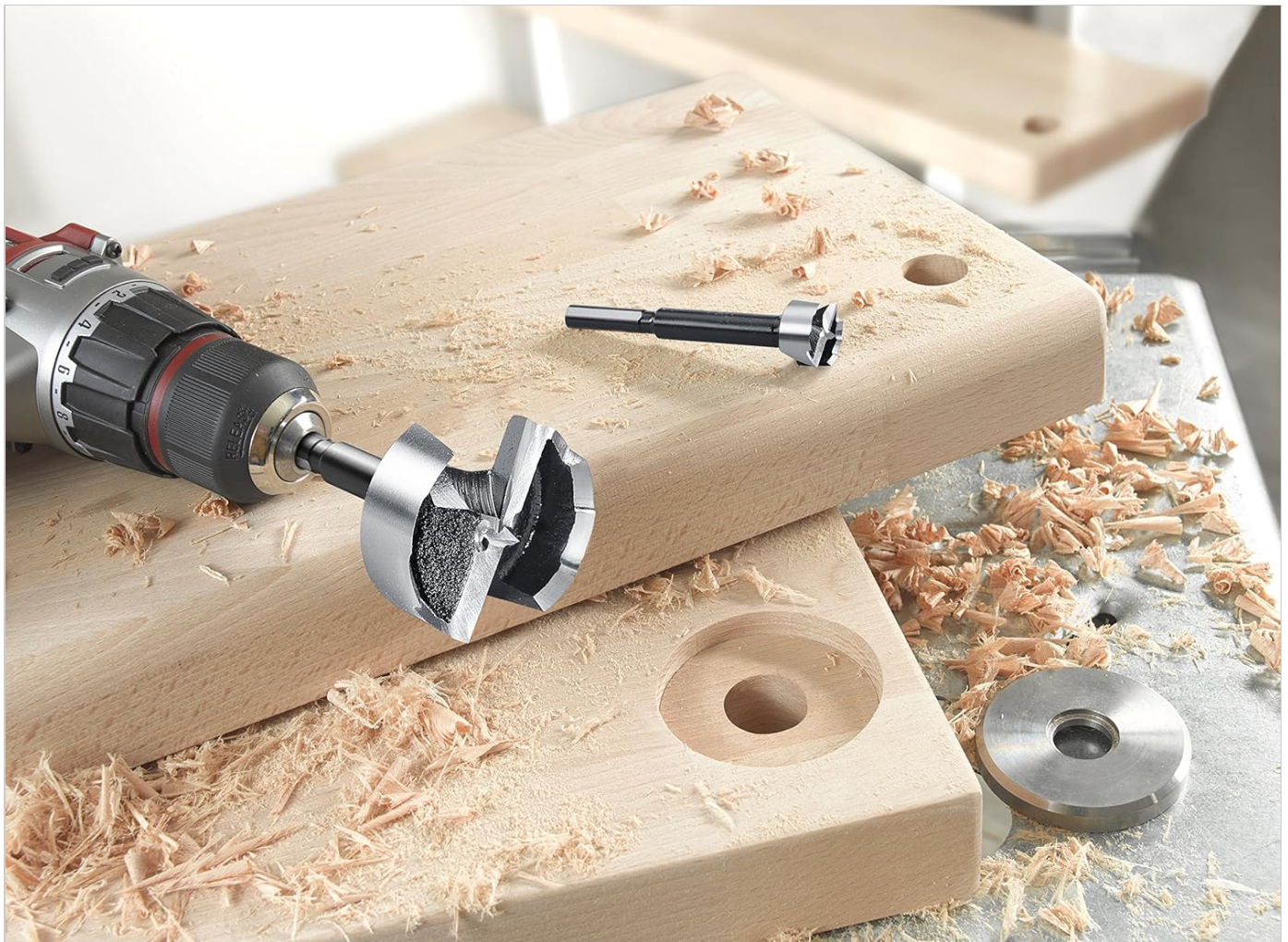
Figure 4: Example application: using the Forstner bit to create a hole for cable management in a desk.
