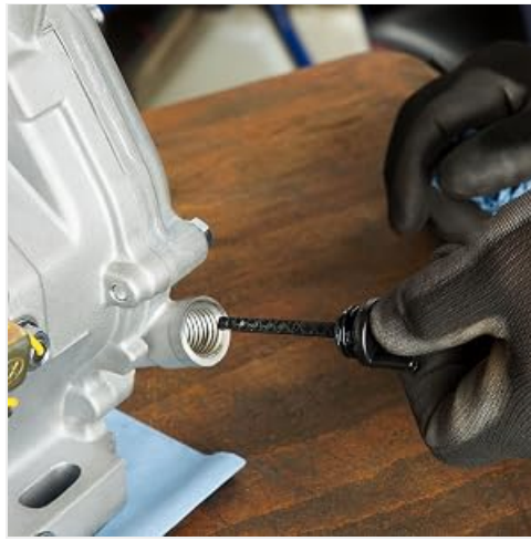
Figure 3: Illustration of checking and filling engine oil.
