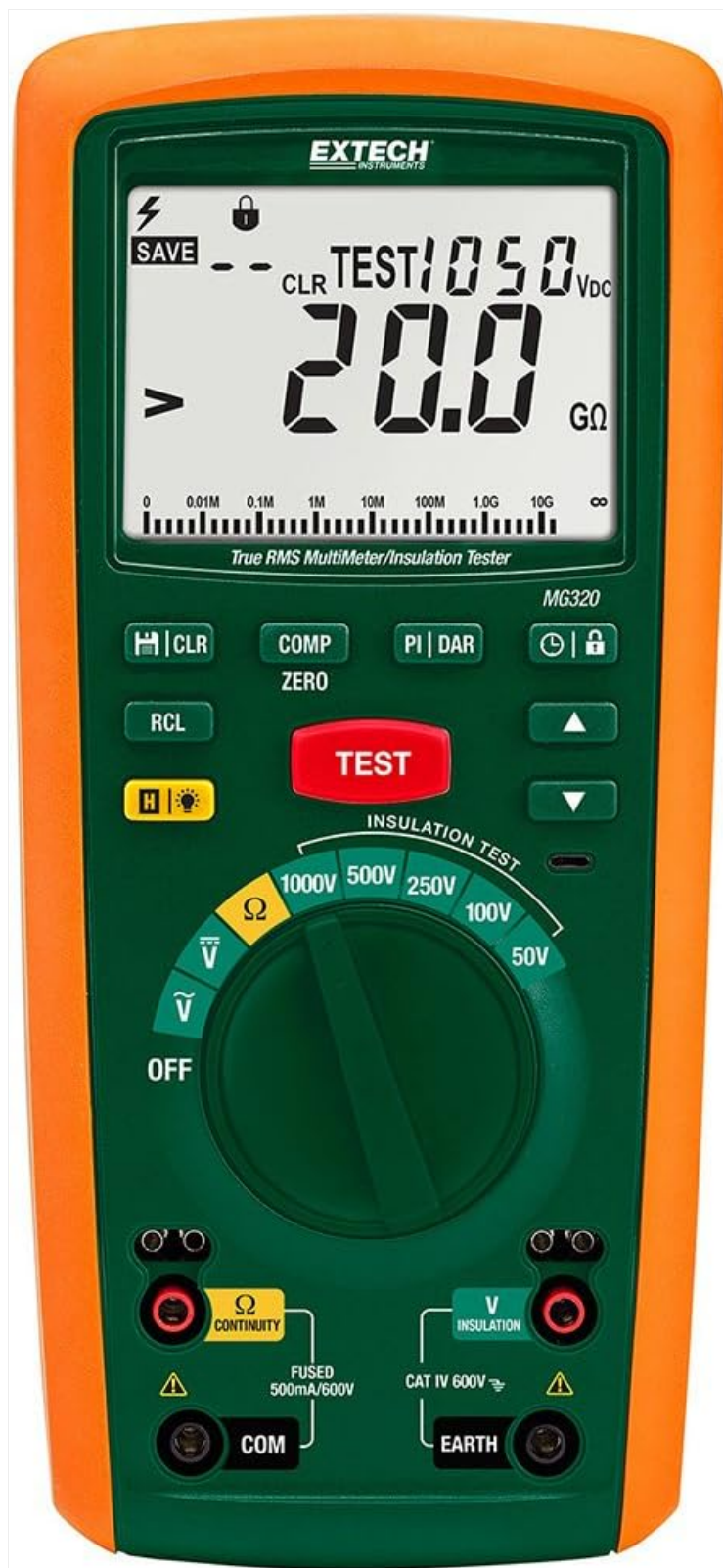
Figure 1: Front view of the Extech MG320 Insulation Tester, showing the display, function dial, and input terminals.
