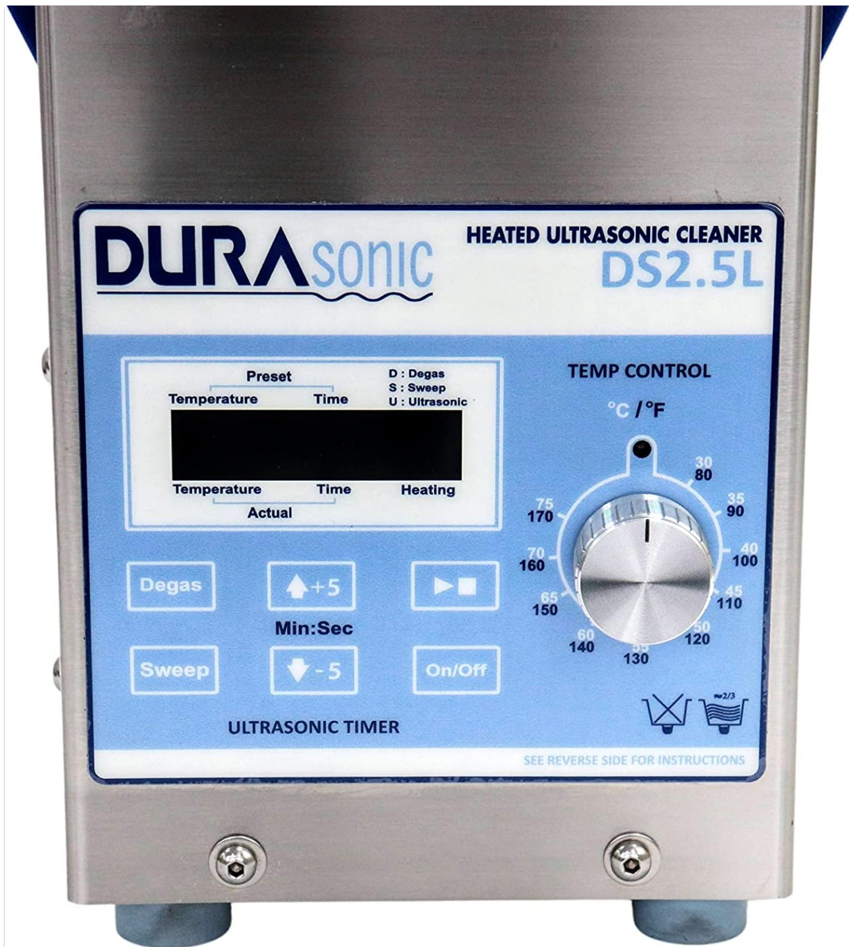
Figure 4.2: Detailed view of the control panel, showing the display, temperature knob, and function buttons.
