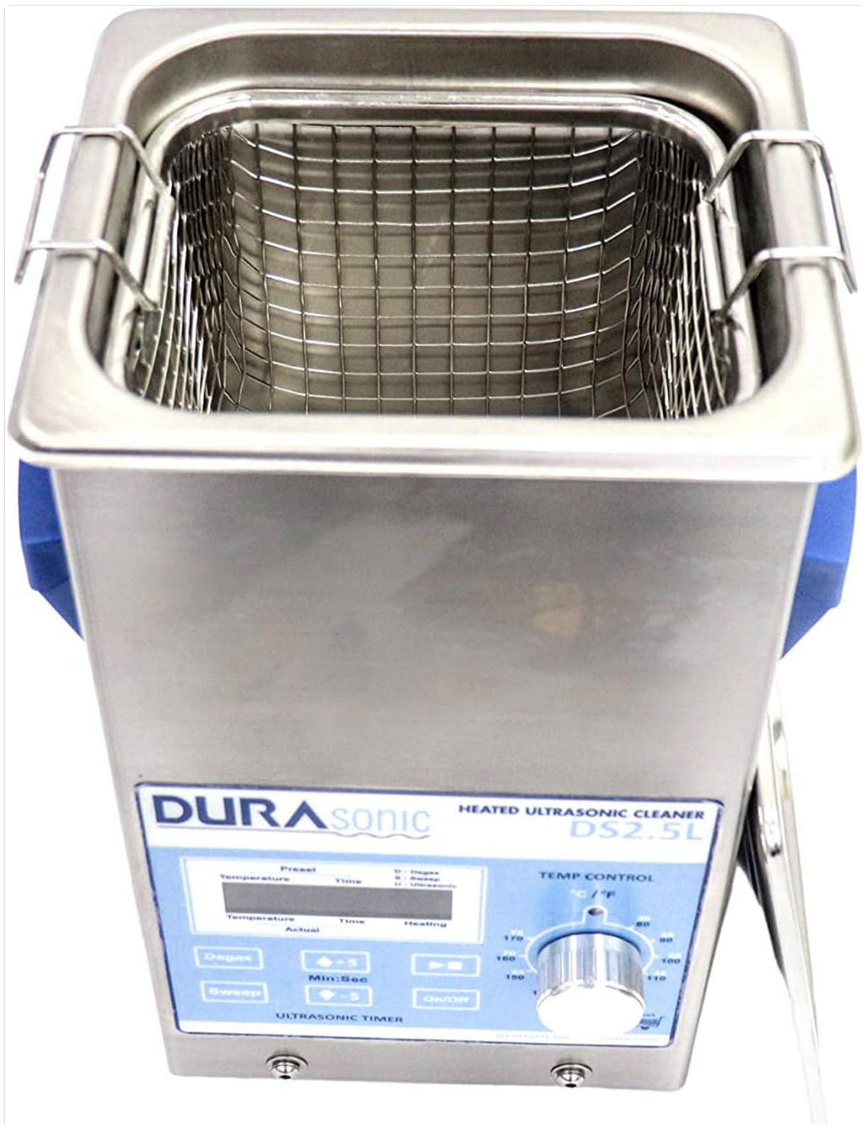
Figure 5.1: Top-down view showing the cleaning basket properly placed inside the tank, submerged in solution.
