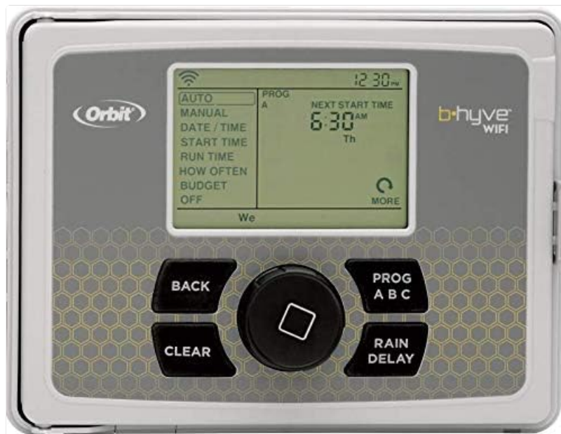
Close-up view of the Orbit B-Hyve controller's front panel, showing the LCD display, navigation buttons (BACK, CLEAR, PROG A B C, RAIN DELAY), and the central control dial. This details the physical interface for direct control.
