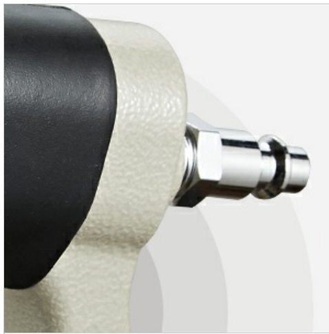
Figure 3.1: The 1/4" NPT air inlet for connecting the air hose to the P515 tool.
