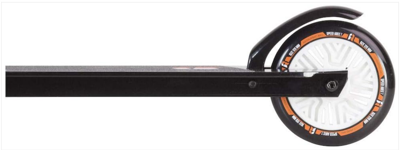
Figure 5.1: A detailed view of the rear wheel and fender brake system. Regular inspection of this area is vital for safe operation and effective braking.
