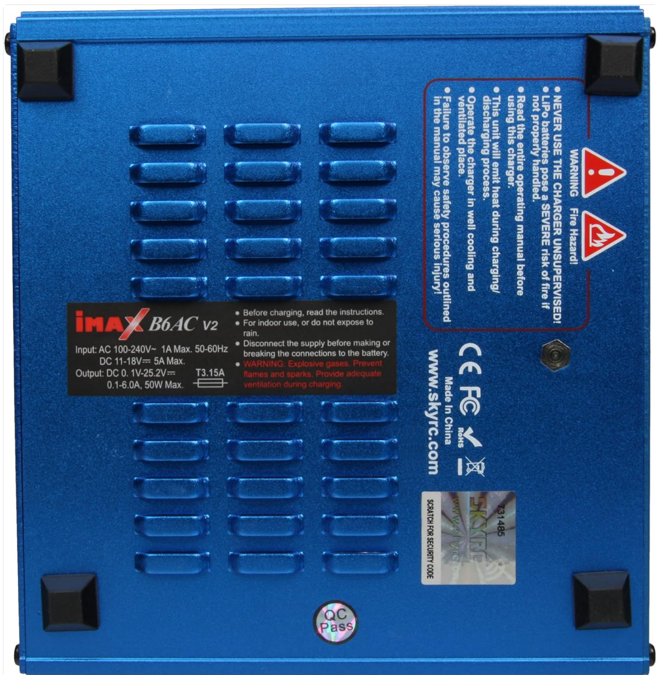
Image: Bottom of the charger displaying critical safety warnings and input/output specifications. Note the fire hazard symbol and warnings about unsupervised use and LiPo battery risks.
