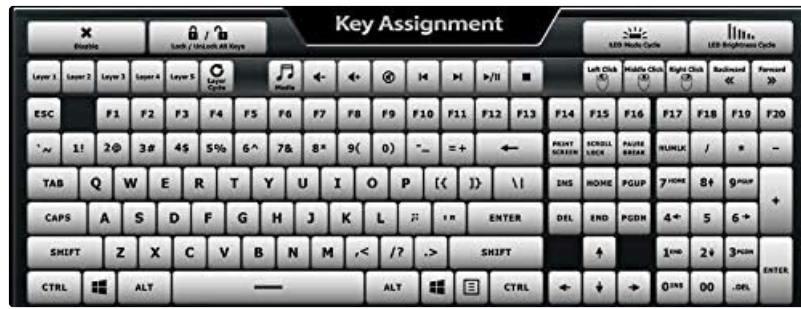
Figure 4: Detailed Key Assignment screen, offering a wide range of keyboard, mouse, and multimedia functions to assign to each key.
