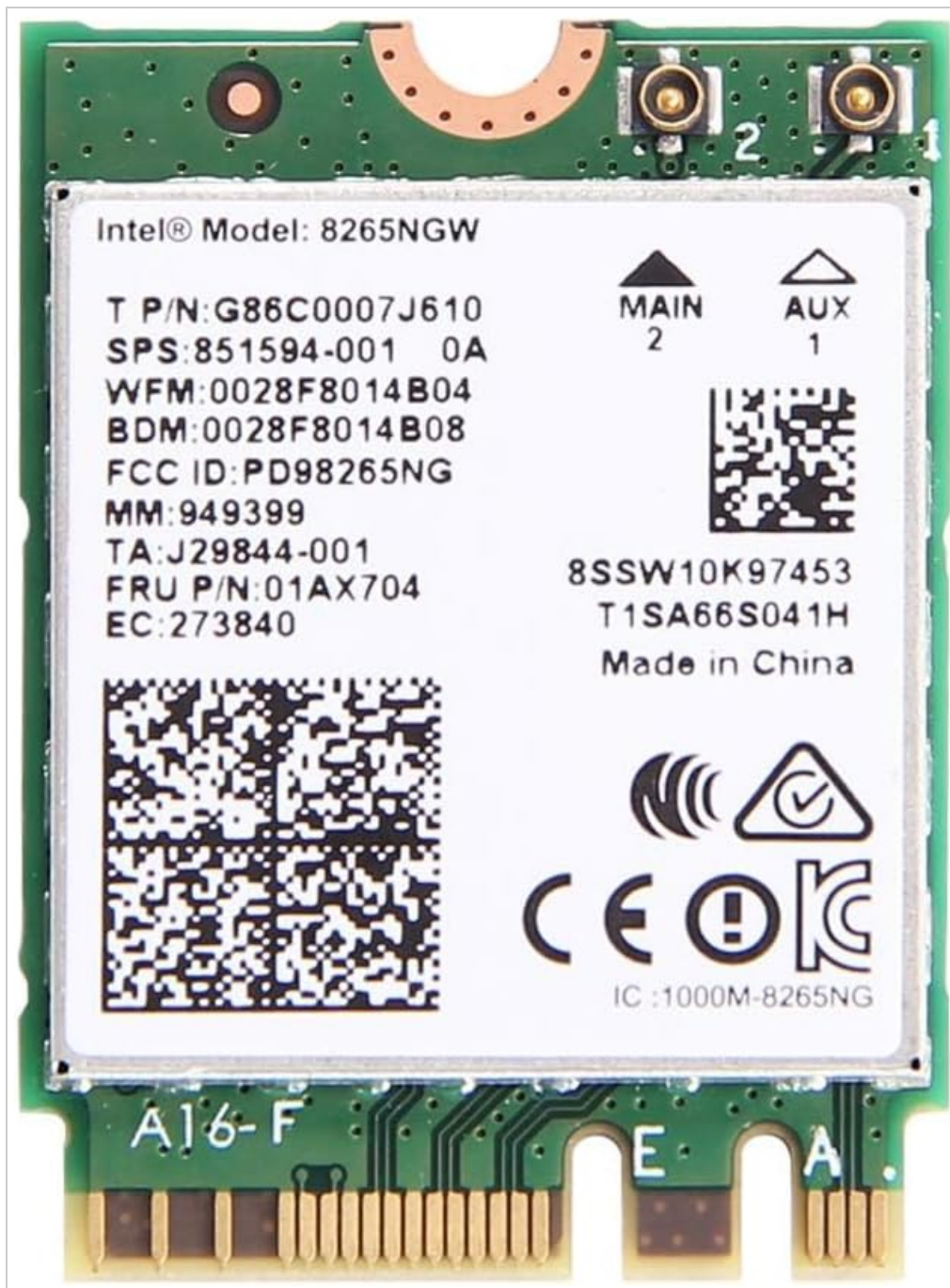
Figure 1: Front view of the Siren Dual Band Wireless-AC 8265NGW M.2 NGFF Wi-Fi Card, showing the Intel 8265NGW model number and various regulatory markings.
