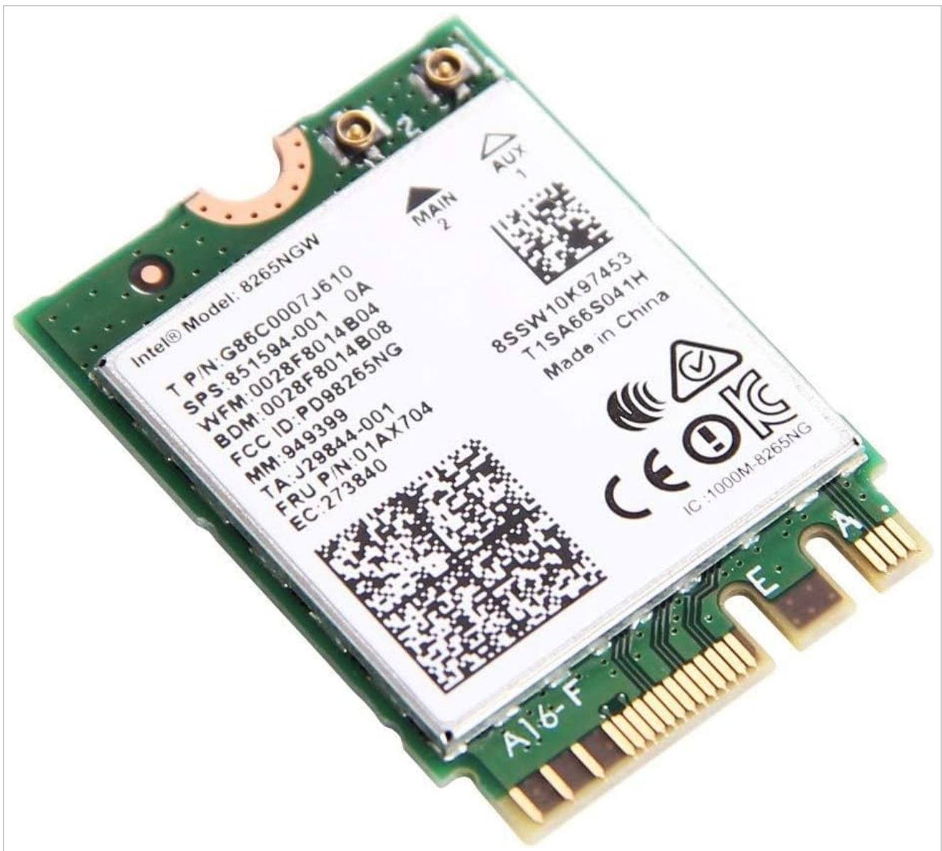
Figure 2: Angled view of the Siren 8265NGW card, highlighting the M.2 connector and the two antenna connection points (MAIN and AUX).
