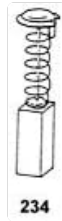
Image 4.1: Schematic diagram illustrating a carbon brush assembly with its spring and cap.
