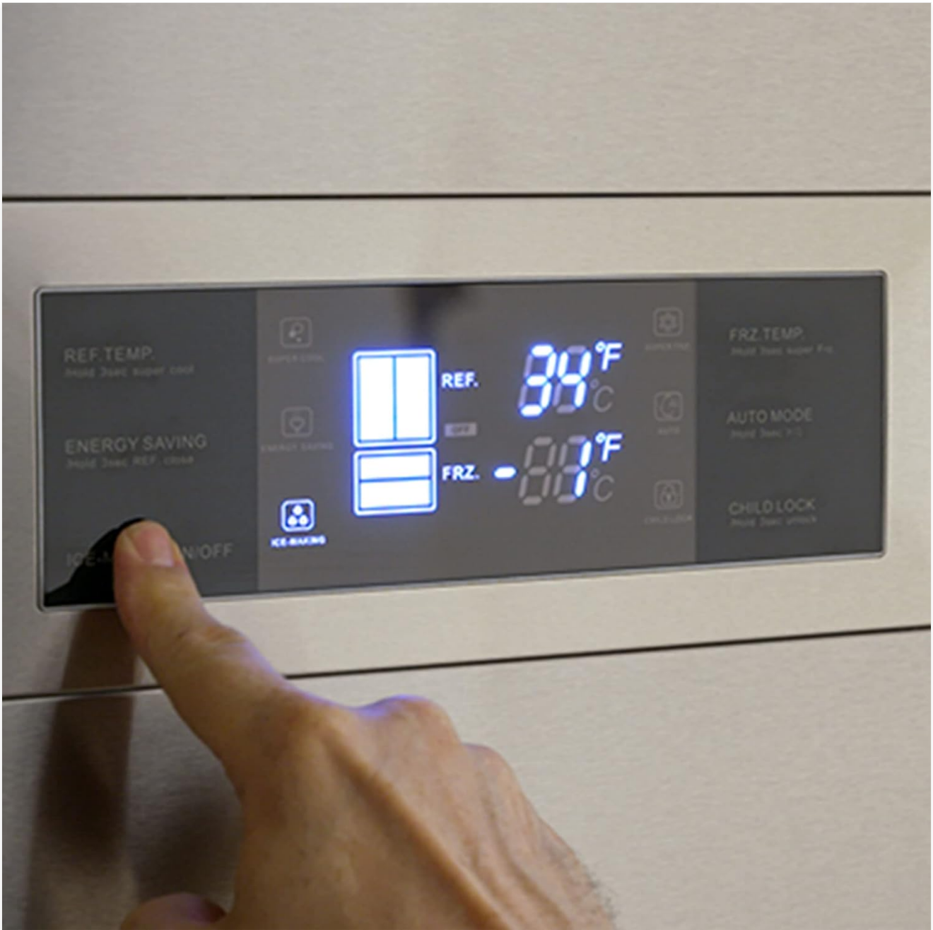
Figure 3: Refrigerator Control Panel.
