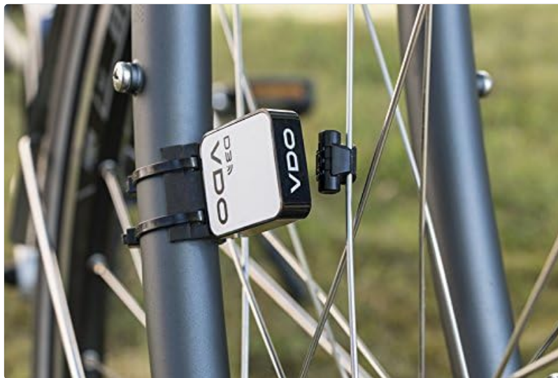
Figure 3: The speed sensor and wheel magnet installed on the bicycle's front fork and wheel.
