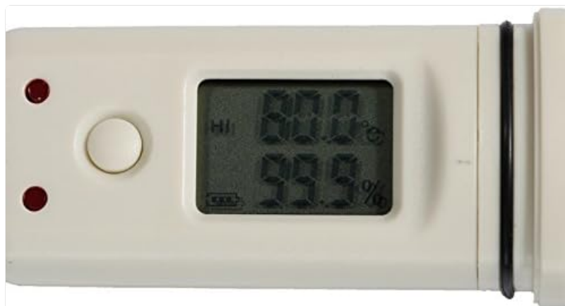
Figure 5: The LCD display showing temperature and humidity readings, along with battery indicator.
