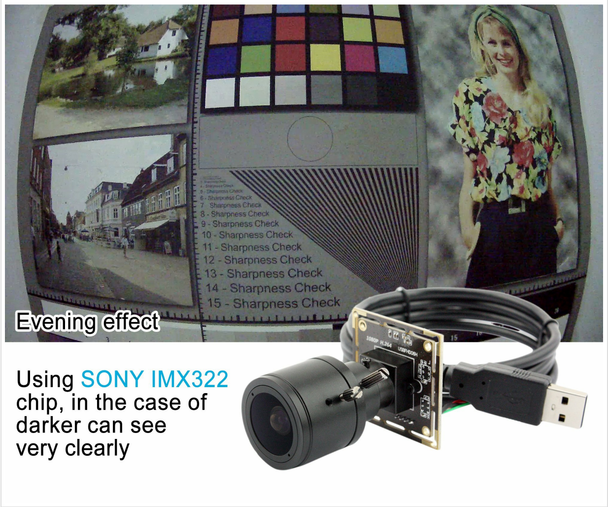
Figure 5: Low illumination performance with Sony IMX322 sensor.
