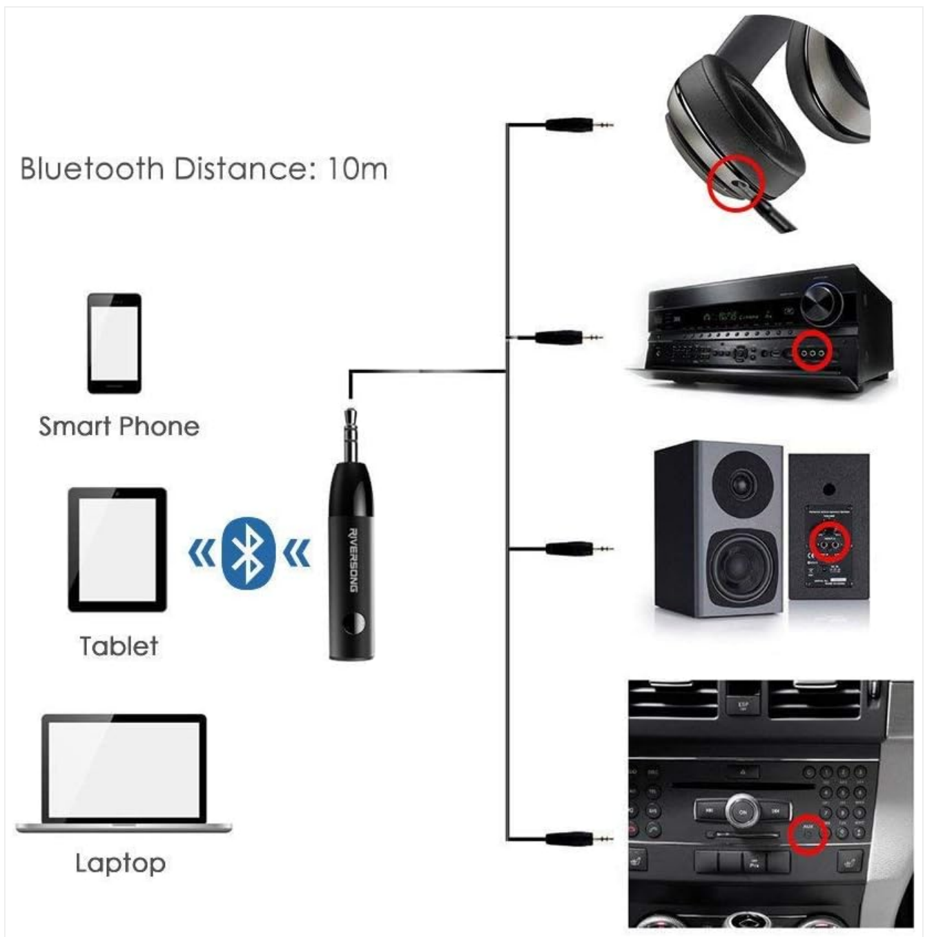
Image 5.2.3: Connectivity diagram showing the RIVERSONG Bluetooth Adapter as a central hub, wirelessly receiving audio from smartphones, tablets, or laptops, and outputting it via 3.5mm to headphones, home audio receivers, standalone speakers, or car auxiliary inputs.
