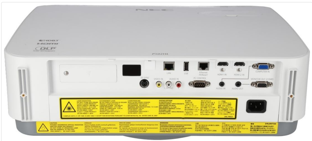
Figure 2: Rear view of the NEC P502HL-2 DLP Projector, highlighting various input/output ports and important safety warning labels regarding laser radiation.
