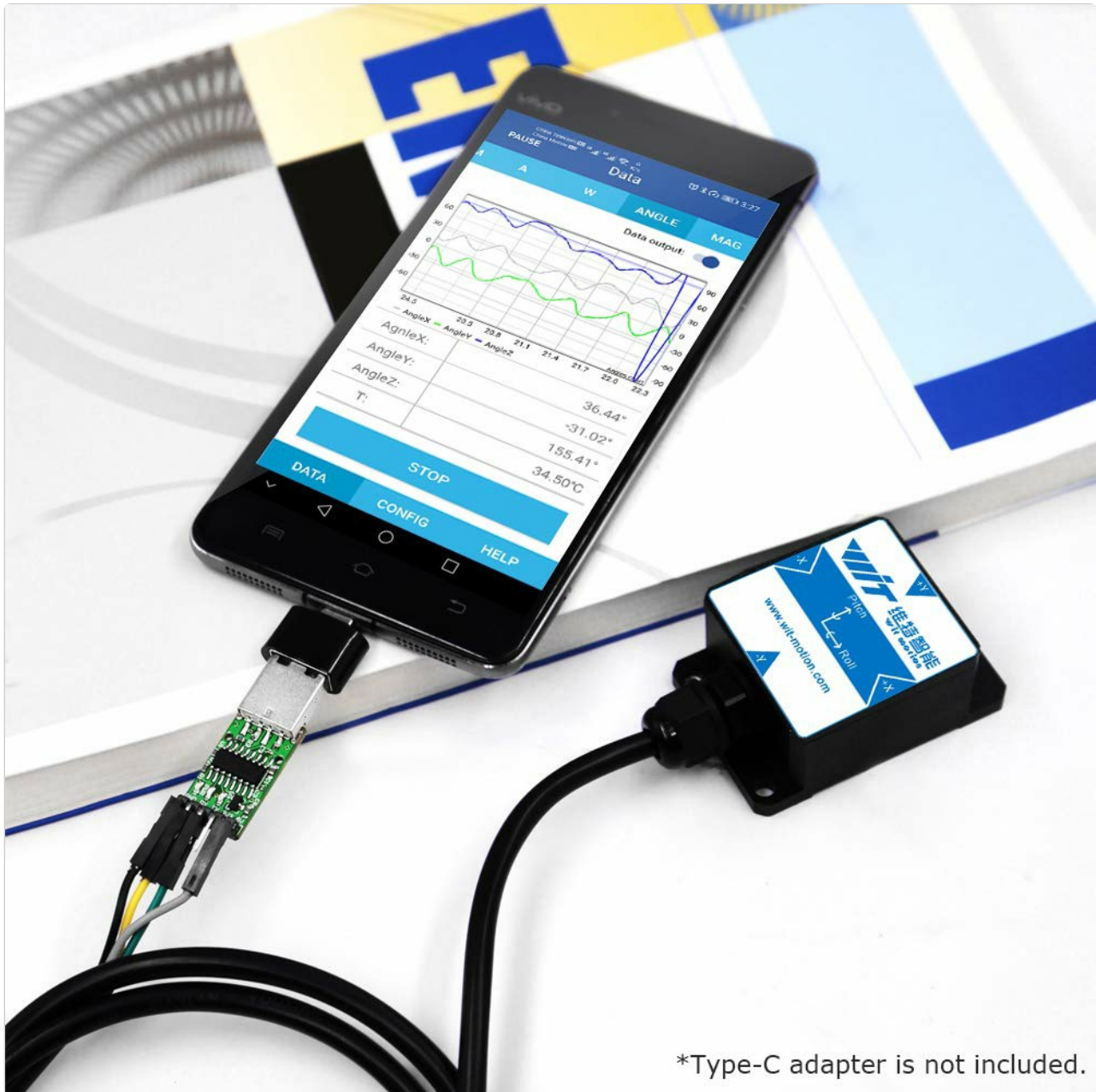
Figure 5.2: The HWT901B-TTL connected to an Android smartphone using a USB-TTL converter and a Type-C adapter.
