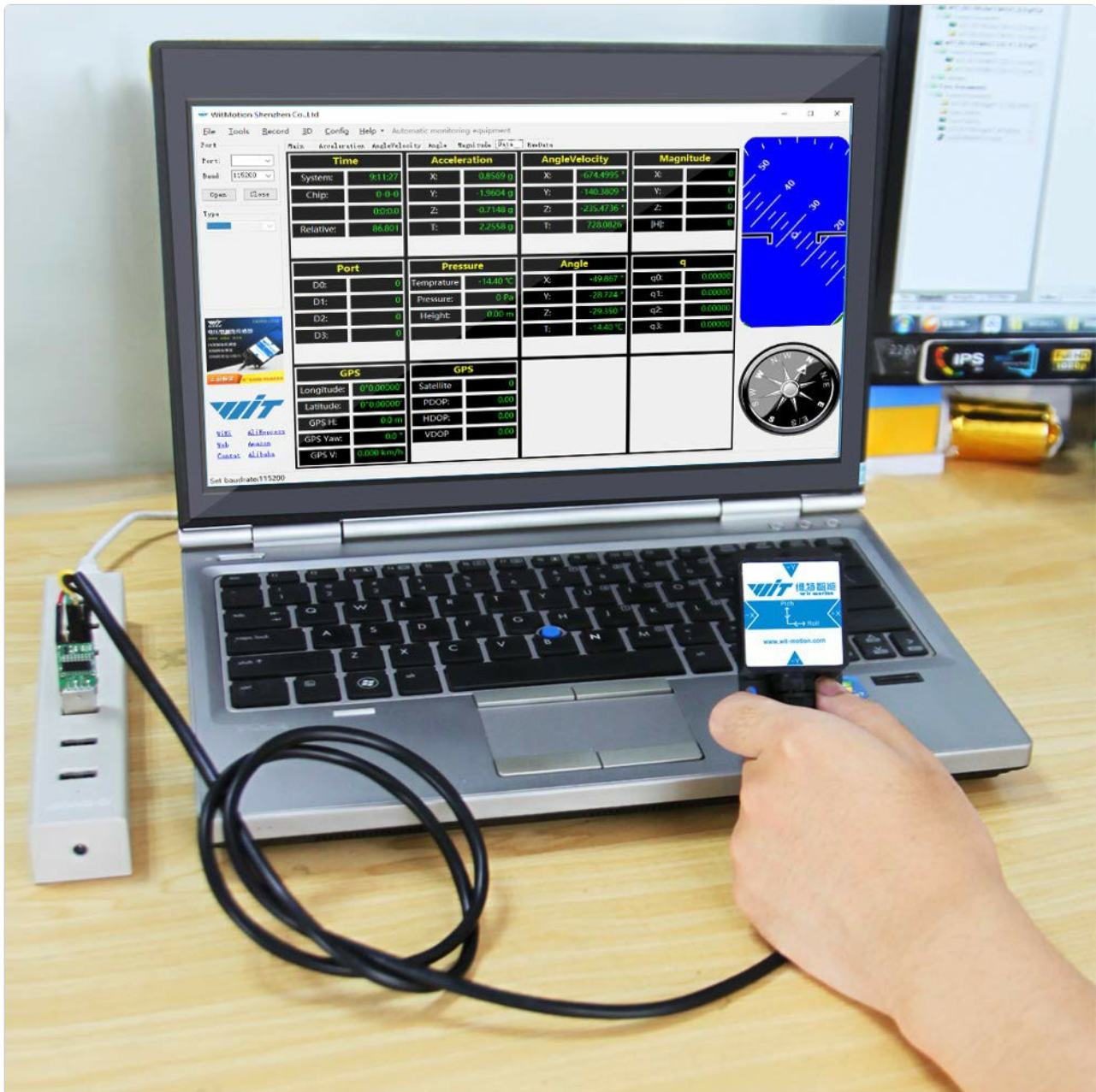
Figure 5.1: The HWT901B-TTL connected to a PC via a serial converter, displaying real-time data on the WITMOTION software interface.
