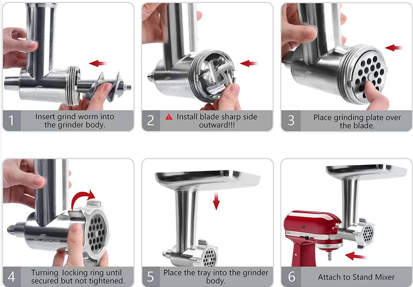
Figure 2: Step-by-step assembly of the meat grinder attachment.
