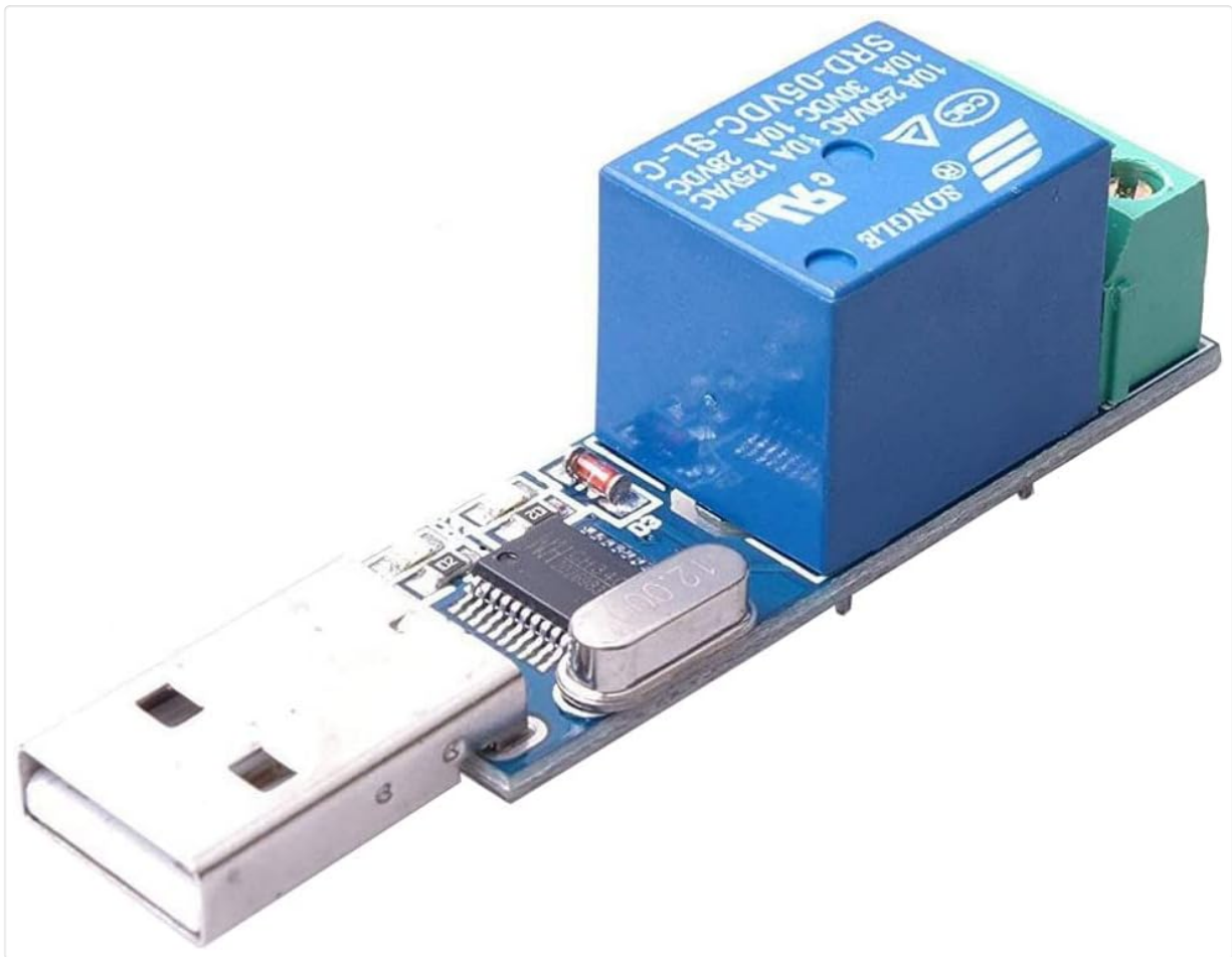
Figure 1: Top-down view of the WINGONEER LCUS - Type 1 USB Relay Module.
