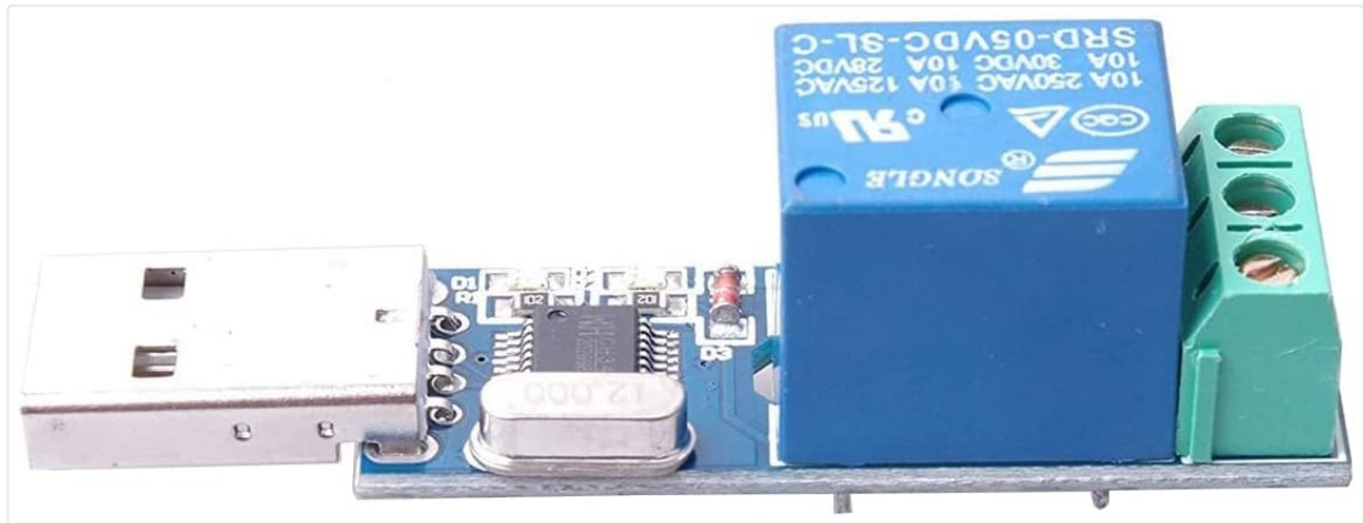
Figure 2: USB connector and CH340 chip on the module.
