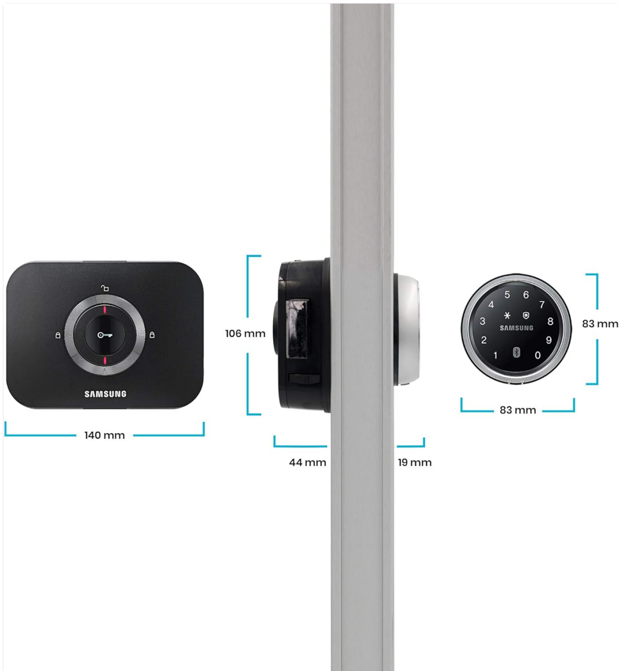
Figure 4.4: Dimensional diagram of the Samsung SHP-DS705 lock. The exterior unit measures 83mm in diameter and 19mm in depth. The interior unit measures 140mm in width and 106mm in height. The total depth of the lock mechanism within the door is 44mm.
